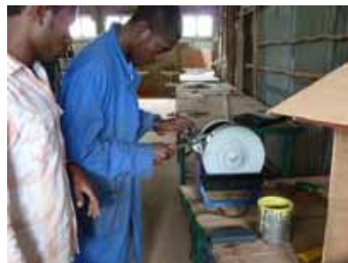
Practising water-cooled grinding
